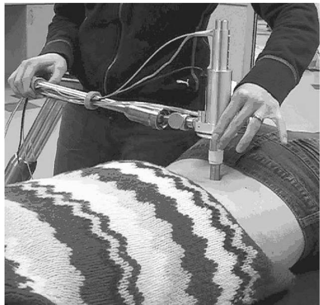
Fig. 2. Placement of the Assisted Indentor on a subject.
